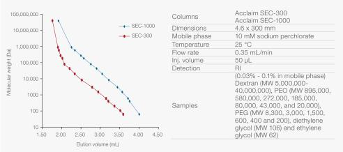
Figure 1: Calibration curves of Acclaim SEC-300 and Acclaim SEC-1000 columns
