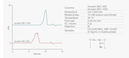
Figure 8: Polyacrylamide CH, CHCONH, on Acclaim SEC-300 vs. Acclaim SEC-1000 columns
