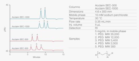
Figure 2: Polyethylene glycols (P'EG) on Acclaim SEC-300 vs. Acclaim SEC-1000 columns
