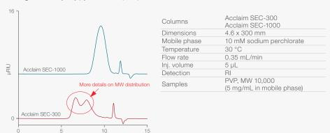
Figure 4: Polyvinylpyrrolidone on Acclaim SEC-300 vs. Acclaim SEC-1000 columns
