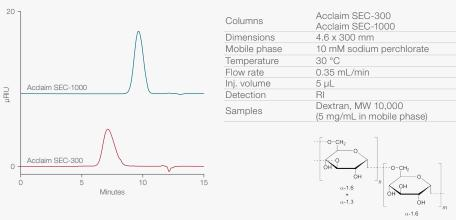
Figure 6: Dextran on Acclaim SEC-300 vs. Acclaim SEC-1000 columns
