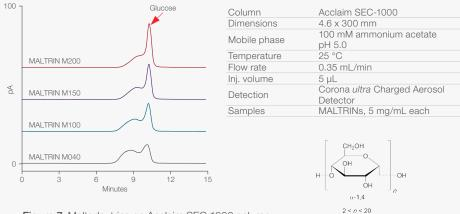
Figure 7: Maltodextrins on Acclaim SEC-1000 column
