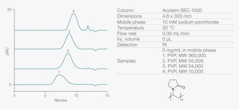
Figure 3: Polyvinylpyrrolidones (PVP) on Acclaim SEC-1000 column
