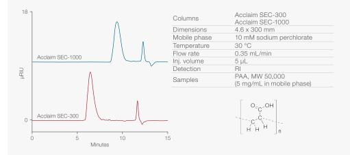
Figure 9: Polyacrylic acid (PAA) on Acclaim SEC-300 vs. Acclaim SEC-1000 columns
